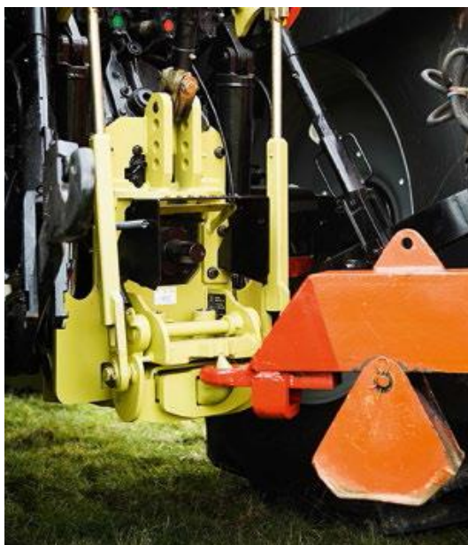
Figure 4: Image of 'hook and ring' type coupling. (Image courtesy of Dromone Engineering).
