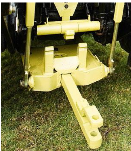
Figure 5: Image of 'pin and eye' type coupling. (Image courtesy of Dromone Engineering).
