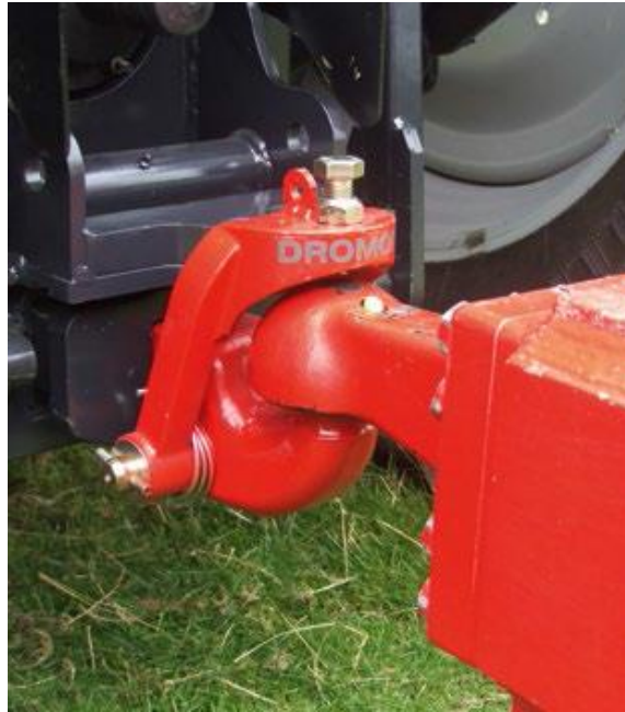
Figure 6: Image of 'ball and spoon' type coupling. (Image courtesy of Dromone Engineering).
